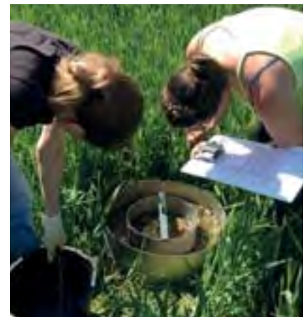
Double ring infiltrometer in use in an arable field. © Chris Stoate/GWCT
